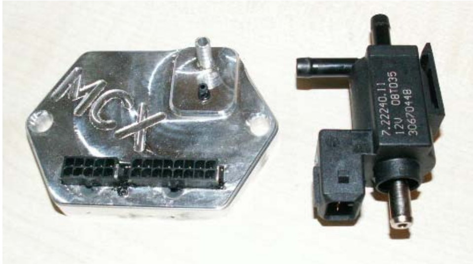
The intelligent EFI-box and the TCV-valve that controls the turbo pressure.
